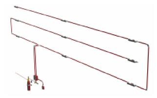
It can be installed as a simple detection (TK-SIMPLEX: positive on one line) or crossed (TK-COMPLEX: need positive crossed lines), with thermal fuse calibrated at different temperatures of action.
